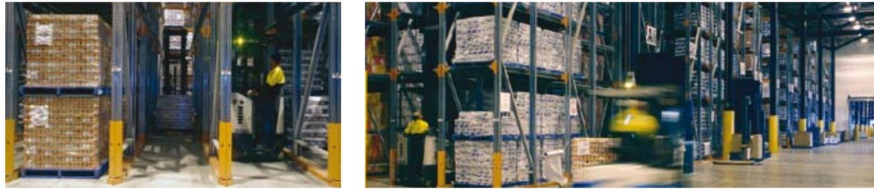
Drive-In pallet racking is the lowest cost and most popular form of high density pallet storage. Drive-In racking provides excellent storage capacity in applications where there is a large quantity of pallets for each SKU. It is ideal for many industry sectors including general manufacturing, food and beverage as well as the cold storage industry.
